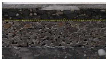
Figure 14 – no material displacement between surface layer and PUR interlayer
