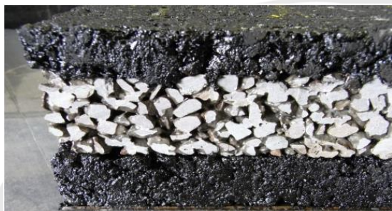
Figure 5 – test specimen with PUR-interlayer (detail)
