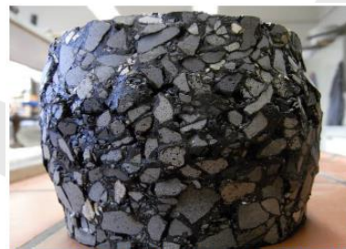
Figure 18 – Visual appearance of the PA interlayer test specimen after the test
