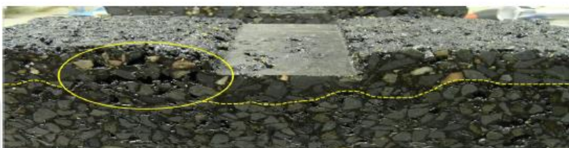
Figure 16 – structural disintegration within the asphalt construction after the test – PA interlayer
