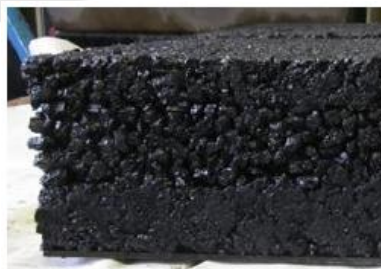
with bituminous interlayer PA 8
