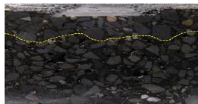
Figure 15 – displacement between surface layer and PA interlayer
